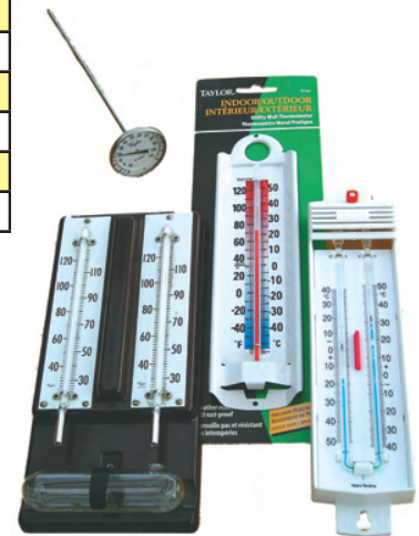
(Top Left) Soil Thermometer (Left to Right) Humidiguide, Greenhouse Thermometer, Max/Min Thermometer
